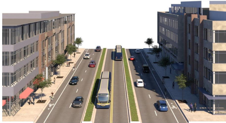
Figure 4-5: LPA Runningway Concept - West Dearborn to Metro Airport (Mixed Traffic Running)
