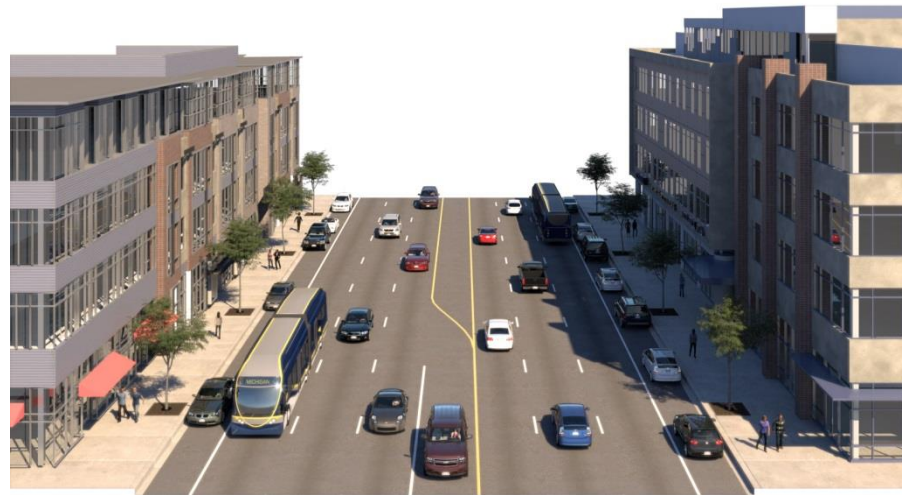
Figure 4-5: LPA Runningway Concept - West Dearborn to Metro Airport (Mixed Traffic Running)
