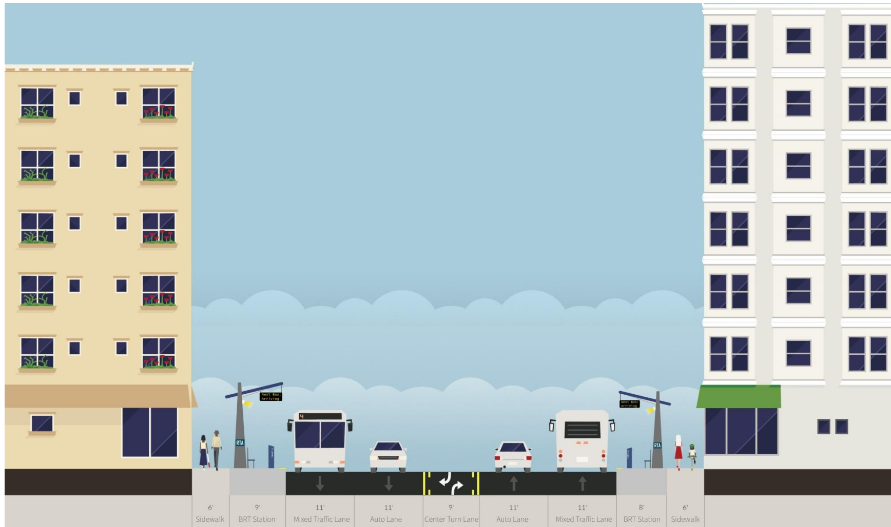
Figure 1-7: LPA Runningway Concept Cross Section - Washtenaw Avenue
