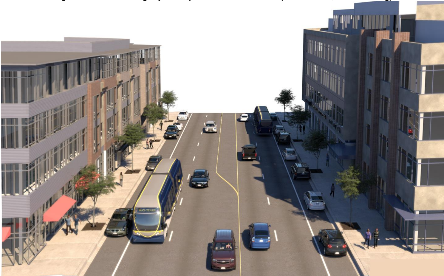
Figure 1-6: LPA Runningway Concept - Washtenaw Avenue (Mixed Traffic, Curb Running)
