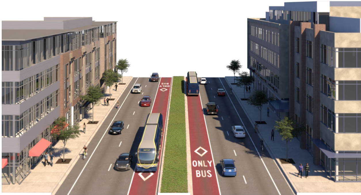
FIGURE 3-10: DEDICATED LANE MEDIAN RUNNING BRT
